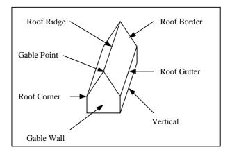
Figure 9. Conceptual feature and structures for a gabled roof
