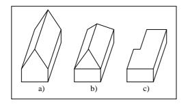
Figure 8. Building roof styles: a) gable, b) hip and c) flat
